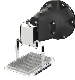
Fig. 3. The CrocoGrip was designed as a general-purpose sterile laboratory gripper for tissue engineering to minimize contamination risks from particles. Its compliant mechanism ensures low particle generation, while maintaining easy cleanability and sterilizability—even for non-experts [2]
